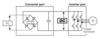
The AC input is first converted to DC by the "Converter "section. Further this DC is then inverted to AC by the "Inverter "Section to supply the desired variable frequency.
