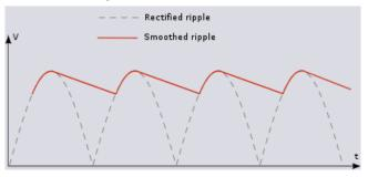
This capacitor is known as DC Link capacitor and it functions as a short-term current source and sink to limit transient voltages seen by power conversion semiconductor switches and the input DC bus. The most commonly used DC Link capacitors are of two types:
